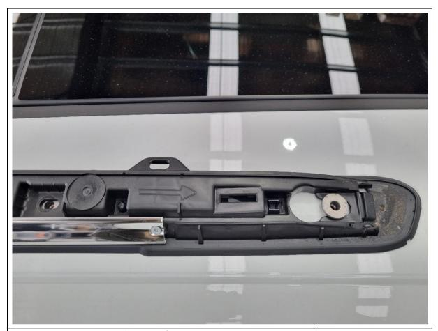
5. Clean out your roof buttons / rivnut threads with a M6 tap to make sure they are clear of residual Loctite that would cause over torque of the rivnut (may even spin it) without achieving the desired rail to rivnut clamping force.
