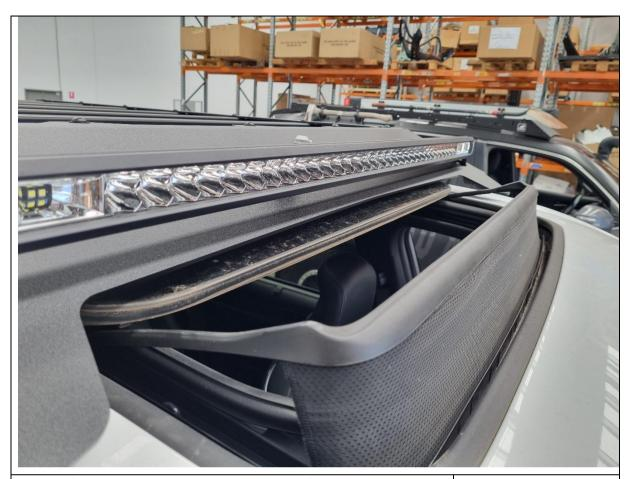
26. If your vehicle is equipped with a sunroof, check to ensure there is clearance to the roof rack in fully open/tilt positions. Adjust the roof rack position fore/aft or up/down with spacer washers if necessary.
