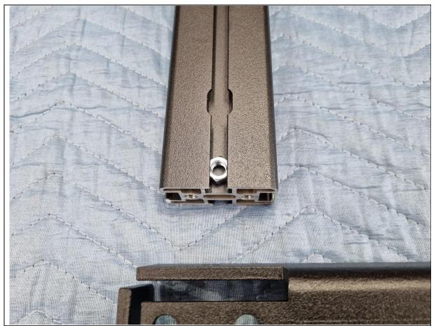
12. Insert 1x M8 nut into the top T-slot of each extrusion end.
