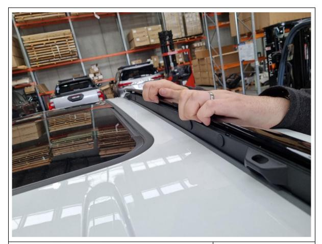
2. Peel off top section of factory rail as shown.
