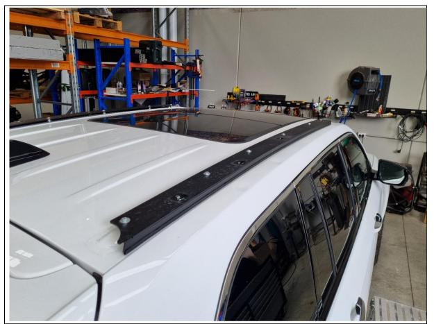
Loosely fit Rails to roof with M6x25 Hex bolts and mud guard washers. Do not torque down yet. 6x per side. Take care not to strip thread and advised to spray WD40 or similar in thread first.
